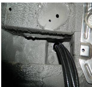
As shown in the figure, the bottom chassis installation crossing point is pierced with a .38 punch and pulled up.
