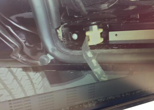
As shown in the figure, the belt transition holes of the 38 reel are drilled. Note: The strap should not touch anywhere.
