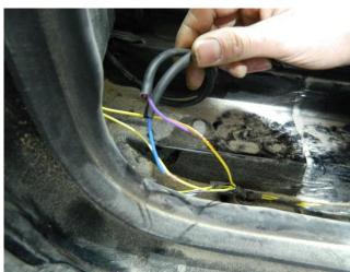
As shown in the figure, the central door control signal (purple cable) in the main system installation will be attached to the yellow red cable found in the original wiring of the vehicle on the B-pillar.
