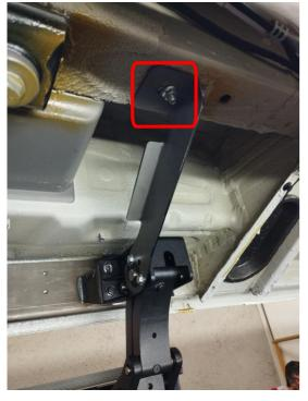
The support legs of the carrier chassis are mounted to the vehicle as shown in the picture.
