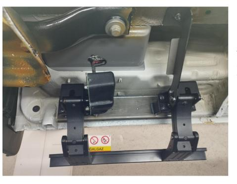
The front connection bolts of the carrier chassis are mounted on the vehicle as shown in the picture.
