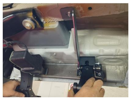
Installation of the rear connecting bolt of the carrier chassis on the vehicle is made as shown in the picture.
