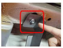
The middle connection bolts of the carrier chassis are mounted on the vehicle as shown in the picture.
