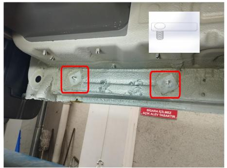
For the carrier chassis connection 3 ps Bolts are placed in the vehicles' original chassis holes.
